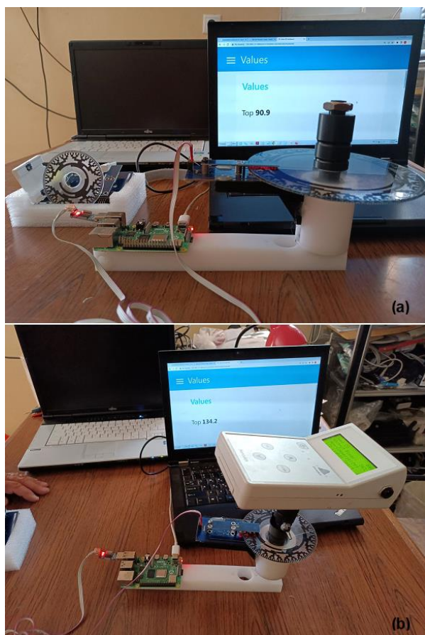
Fig. 2(a): Inertia system sensor, with Gray code disk and data transmission to a computer. It rotates in a circular movement around a vertical shaft. The sensor emits ultra-low (ULF) and very low frequencies (VLF) (3 Hz–30 kHz). (b) The setup showing the sensor, the Raspberry Pi, and the computer connected to them
